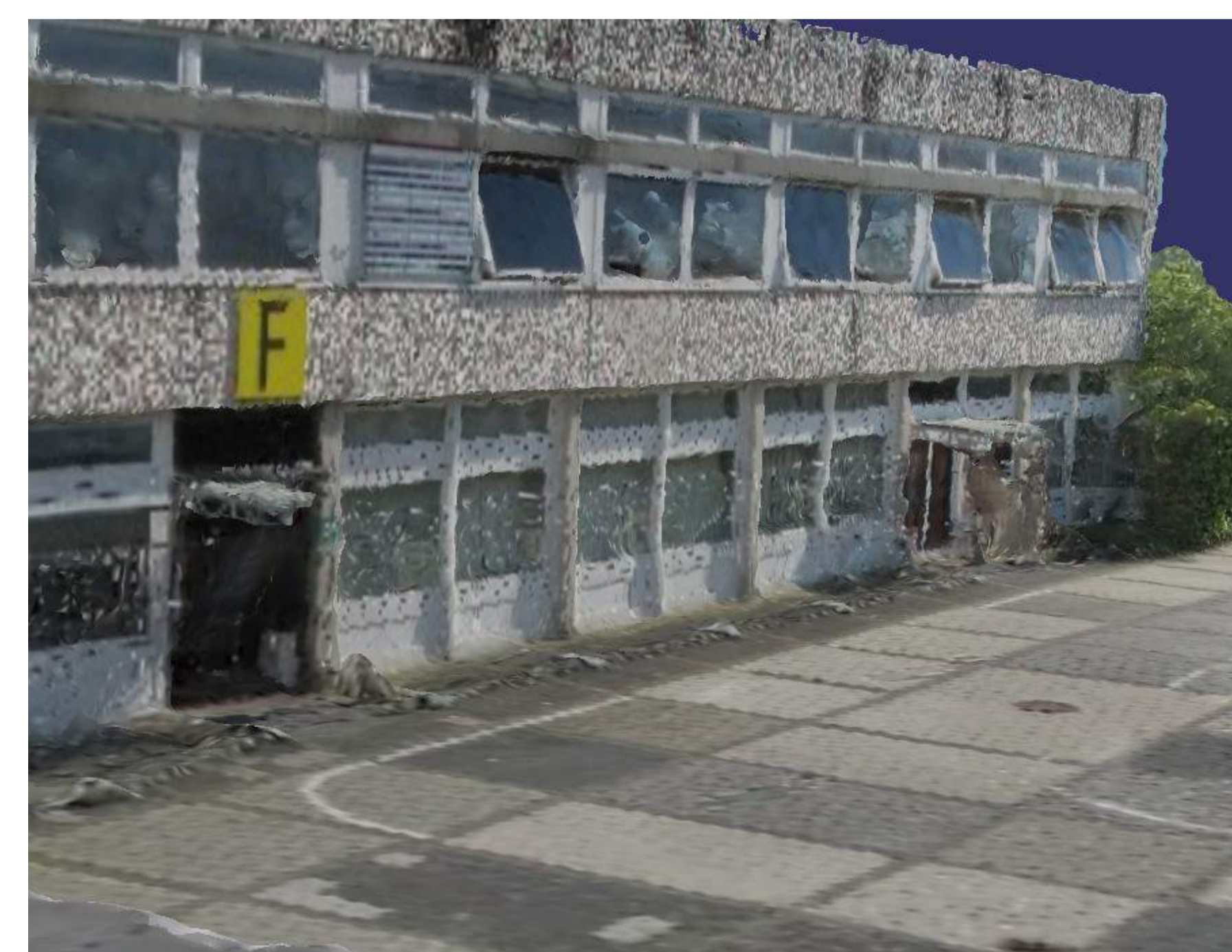
Fusion of airborne and ground pointcloud (with University of Hannover).
