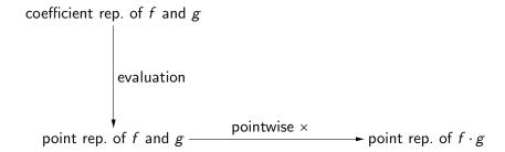
Main principle of the fast Fourier transformation (FFT):
