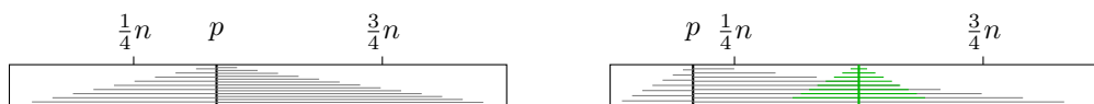
■ Figure 1 Left: A guardian at position p , storing all suffixes of m_1 \dots m_{p-1} and all prefixes of m_p \dots m_n . Right: As soon as p escapes the range [\frac{1}{4}n, \frac{3}{4}n] a new guardian (in green) is started at \frac{n}{2} .
