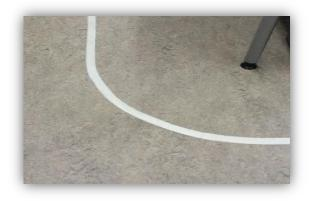
Curve Type: Short Curve Distance: 2.10m Curve Radius: 0.30m
