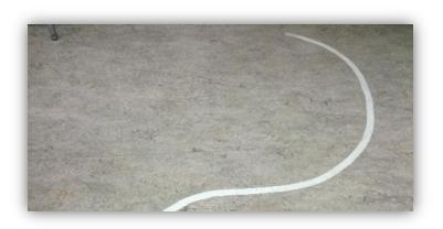
Curve Type: Medium Curve Distance: 1.36m Curve Radius: 0.65m
