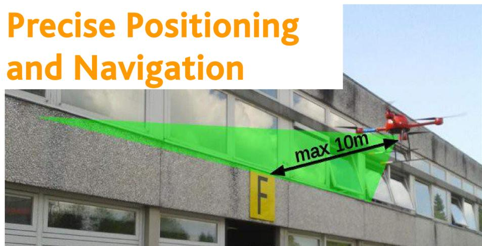
A more precise positioning of UAVs is needed. In addition to the absolute position that is determined by a differential Global Navigation Satellite System (GNSS), the platform is equipped with surrounding sensors (Optical, Ultrasonic, Radar). These assist the pilot in flights next to buildings, walls or other objects and prevent collisions with them.
