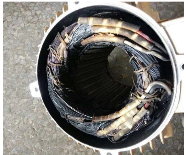
(b) Burned motor windings (source: https://www.simomotor.com )
