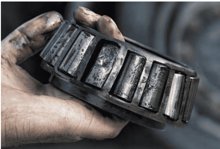
(a) Damaged motor bearing (source: https://renown-electric.com )
