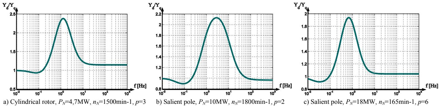
Fig. 2: Frequency dependence of the admittance difference of several machines
