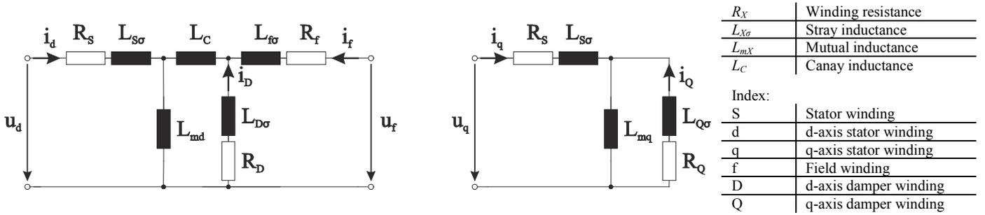
Fig. 1: Equivalent circuit in standstill in d- and q-axes of the SM
