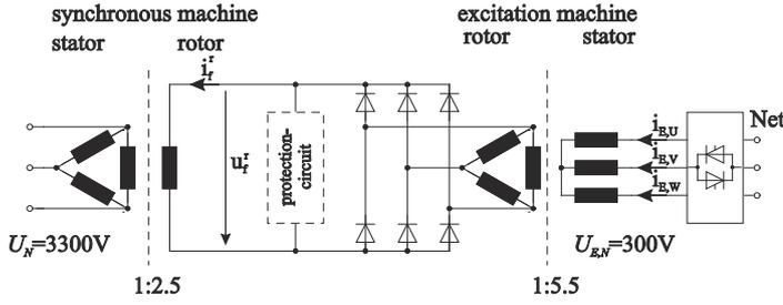
Fig. 3: Winding ratios of a brushless excited synchronous machine
