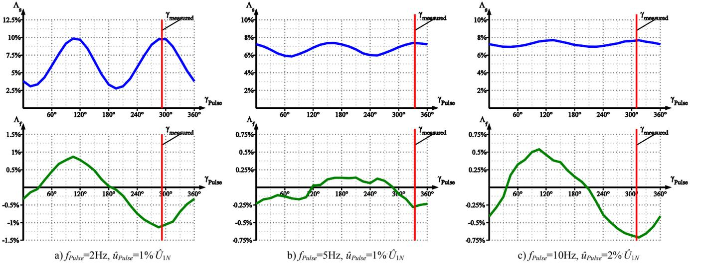
Fig. 6: ID-run with different test signal parameters. (measurement results, 1.1MW Machine, brushless excitation)
