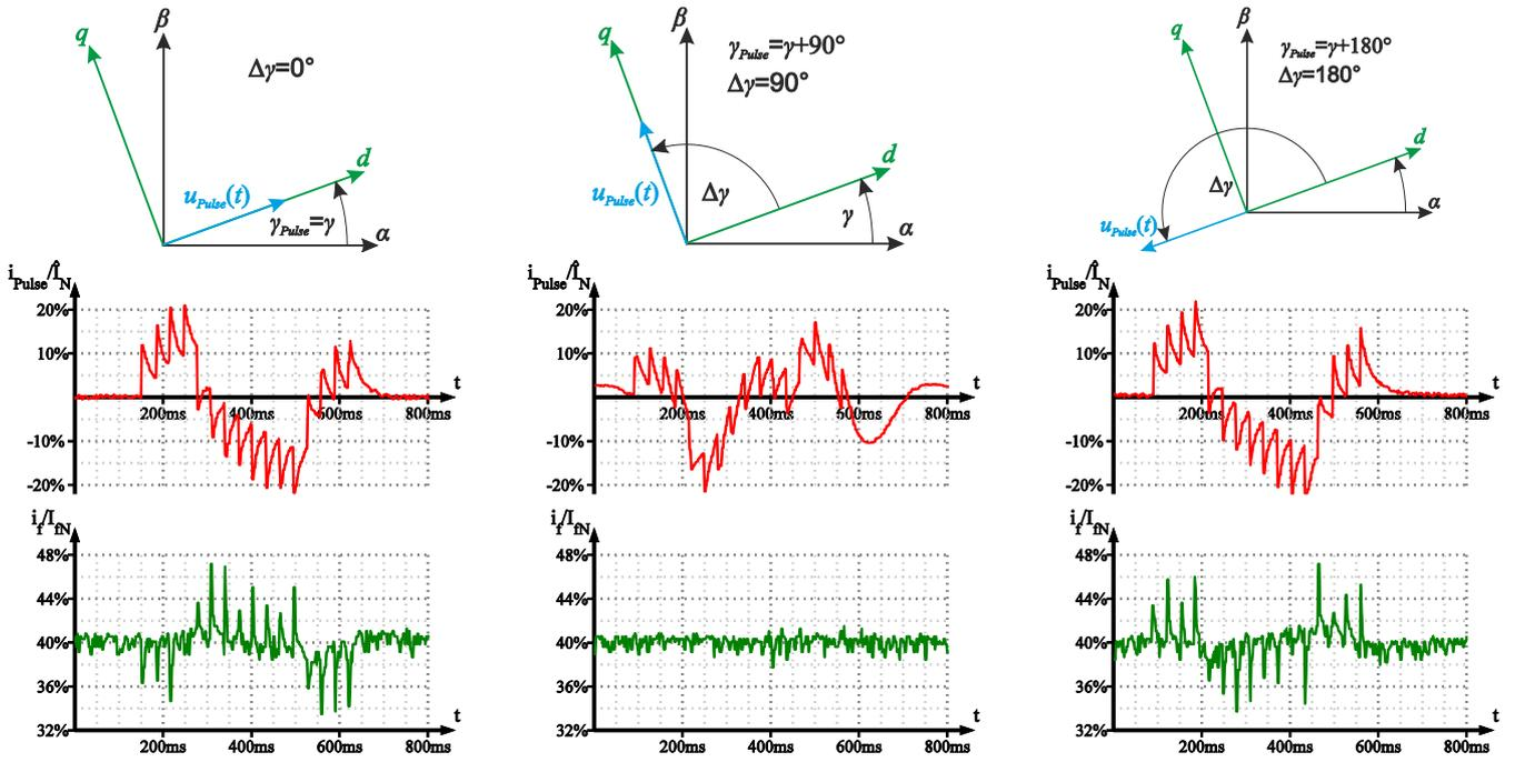
Fig. 5: Test pulse injection in different directions and their current responses (measurement results, 1.1MW Machine)
