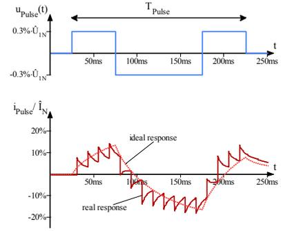
Fig. 4: Stator current response (simulation results)
