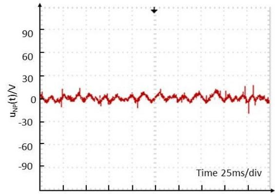
Figure 13. The neutral point voltage for normal D-PWM
