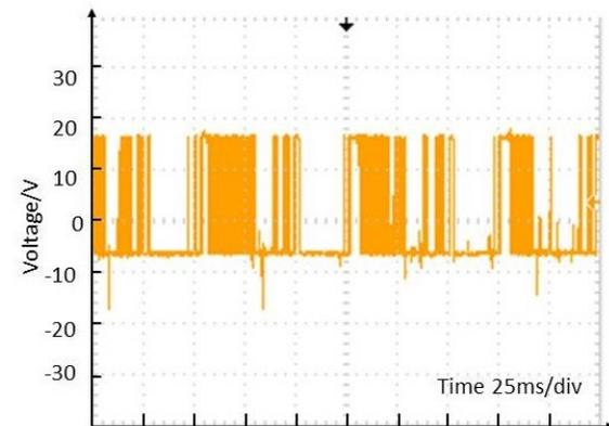
Figure 10. Firing pulses of IGBT 1 for operational map of type A
