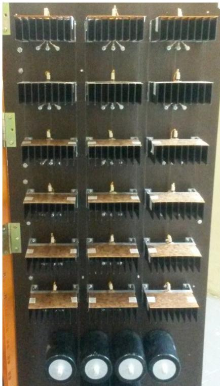
Figure 8. Heat-sinks of the set-up with the 3L-NPC VSI
