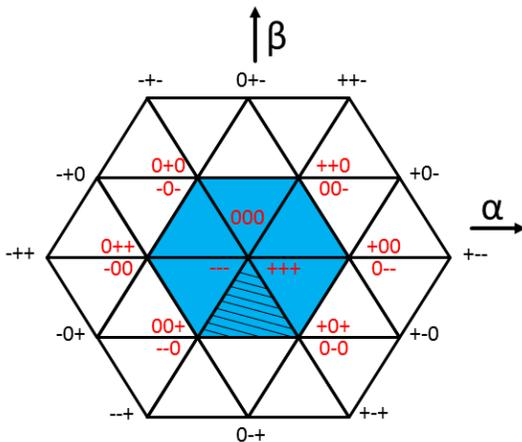
Figure 2. Space vector diagram for a three-level inverter with the redundant states
