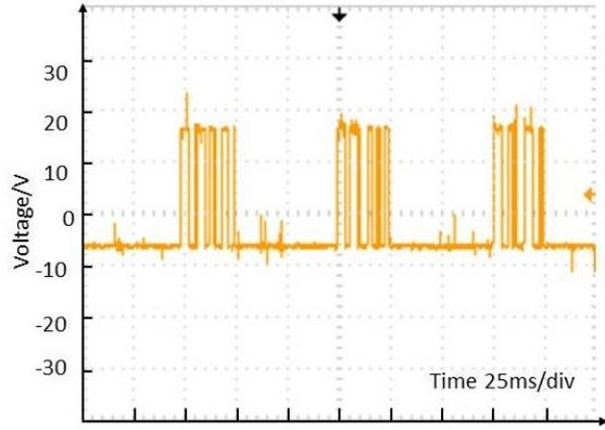
Figure 12. Firing pulses of IGBT 1 for operational map of type C
