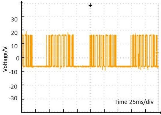
Figure 11. Firing pulses of IGBT 1 for operational map of type B
