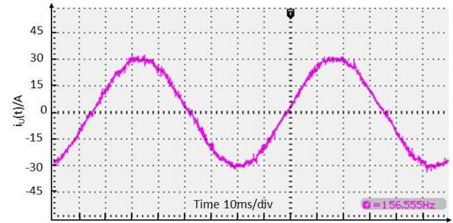
Figure 19. Stator current  $i_u(t)$  for operational map type B
