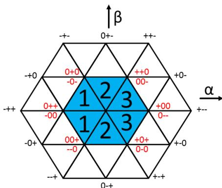
Figure 4. Exclusion of inappropriate switching vectors for reducing the losses of the upper leg of phase U
