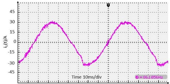
Figure 18. Stator current  $i_u(t)$  for operational map type A
