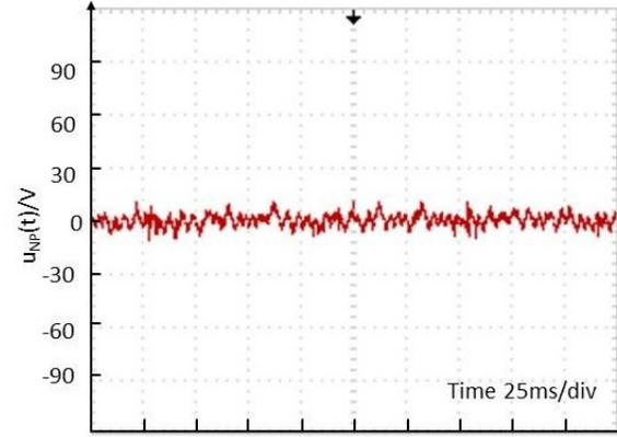
Figure 15. The neutral point voltage for operational map type B
