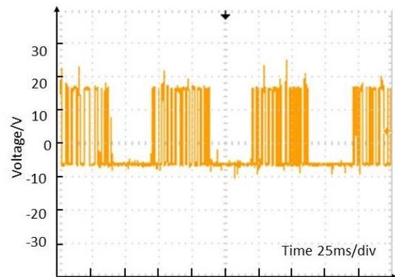
Figure 9. Firing pulses of IGBT 1 for normal D-PWM
