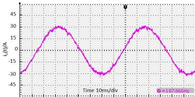
Figure 17. Stator current  $i_u(t)$  for normal D-PWM
