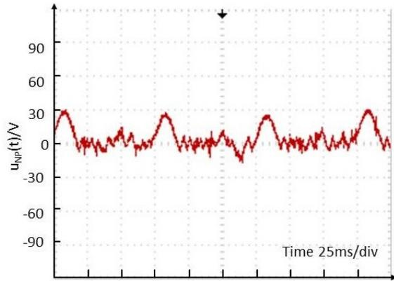
Figure 16. The neutral point voltage for operational map type C
