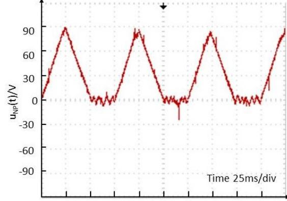
Figure 14. The neutral point voltage for operational map type A
