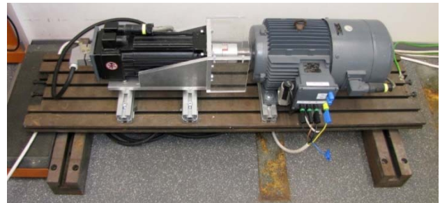
Fig. 5 The utilized PMSM can be seen on the left, the induction machine on the right side. The IM is controlled by a frequency inverter according to the performance curves. The PMSM feeds the generated power to the ZSI.
