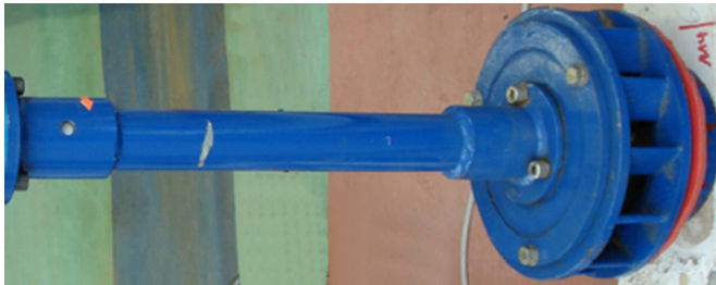
Fig. 2 Low head turbine used as prototype for the measurements in the hydraulic engineering laboratory.
