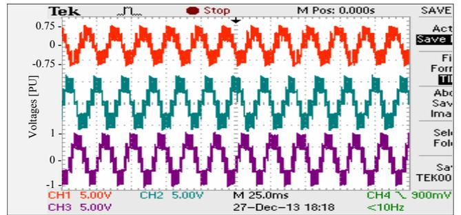
Fig. 10. Total inverter phase voltages with 50% DC-link voltage drift in one cell of phase  $a$  (25 ms/div)
