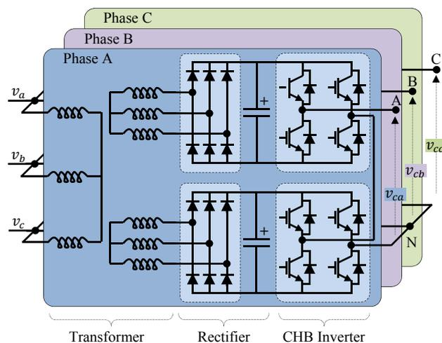
Fig. 1: Proposed system configuration of the 5 level CHB grid connection converter
