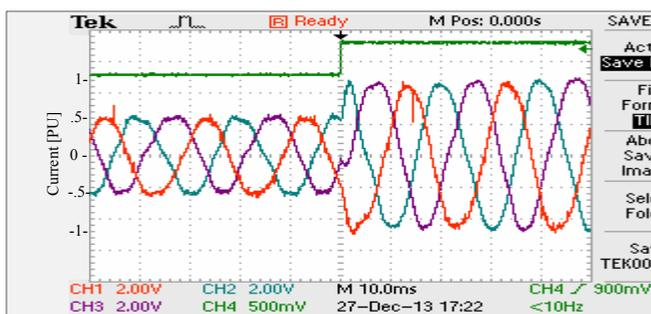
Fig. 9. Inverter current with 50% step change (10 ms/div)
