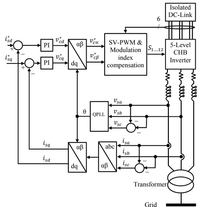
Fig. 2: Control diagram for the CHB converter system
