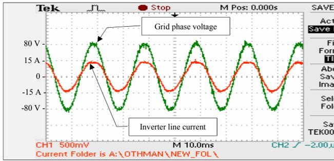
Fig. 7. grid voltage and inverter current in phase  $a$  (10 ms/div)
