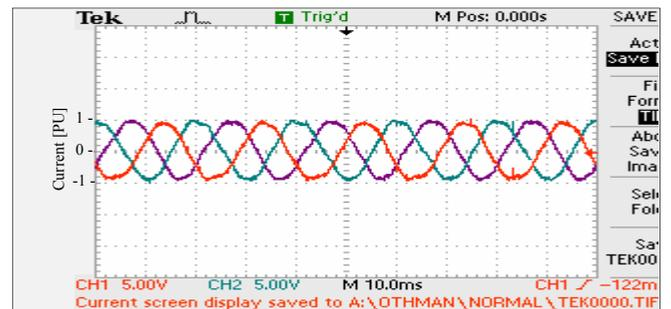
Fig. 6. Inverter currents injected to the grid under normal conditions (10 ms/div)
