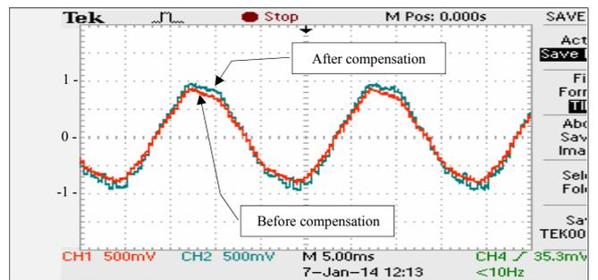
Fig. 12. Modulation index of phase  $a$  before and after compensation (5 ms/div)
