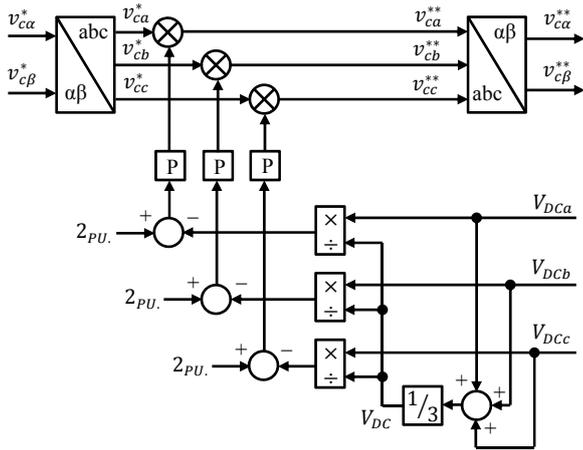
Fig. 3: Feedforward modulation index compensation diagram
