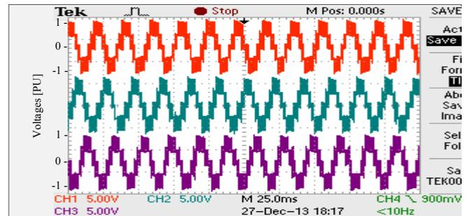
Fig. 5. Total inverter phase voltages under normal condition (25 ms/div)
