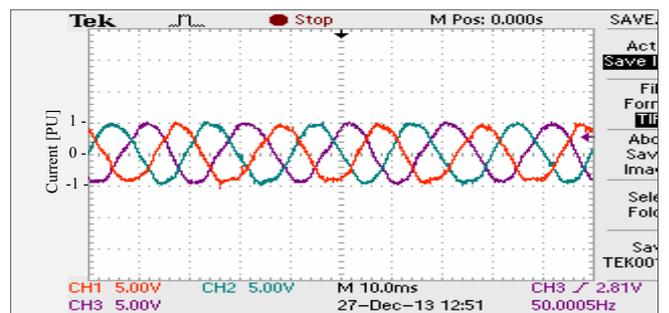
Fig. 11. Inverter currents with 50% DC-link voltage drift in one cell of phase  $a$  (with compensation) (10 ms/div)
