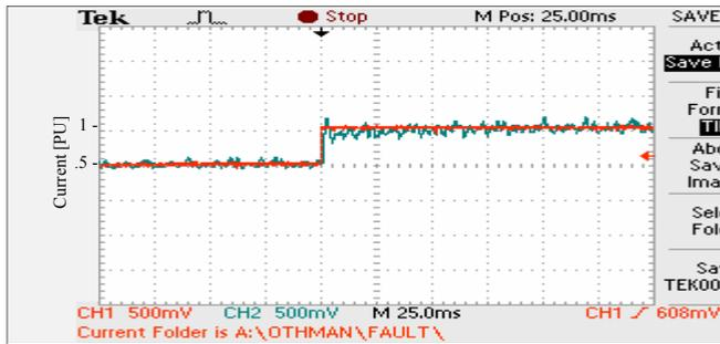
Fig. 8. Refrence current with inverter current step change (25 ms/div)
