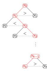
Elements will sink along the path  $[x_0, x_1, x_2, ..., x_{k-1}, x_k]$  which can be computed with only  $\log_2 n$  comparisons.
