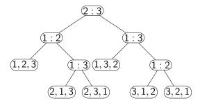
**Note:** The depth (= max. number of edges on a path from the root to a leaf) of the decision tree is the maximal number of comparisons of the algorithm on an input array of length n.
