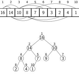
In a first step we will permute the entries of the array  $a[1, \ldots, n]$  such that the heap condition is satisfied.
