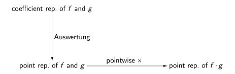
Main principle of the fast Fourier transformation (FFT):
