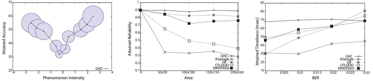
Fig. 6: Top left figure: Impact of phenomenon on attained accuracy, top middle figure: impact of area on attained reliability and top right figure: impact of BER on attained timeliness
