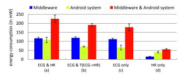
Fig. 10. Energy consumption for different sensor constellations. Having a transformation converting ECG streams to heart rate data (b) saves more than 15 % energy compared to having both sensors connected (a). Compared to an ECG sensor (c), a heart rate sensor (d) consumes perceptible less energy.
