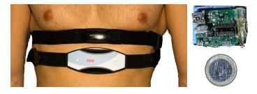
Fig. 6. A Zephyr HxM Bluetooth heart rate sensor and a Corscience CorBELT Bluetooth 1-lead ECG sensor were used for testing the  $T_{ECG \rightarrow HR}$  transformation and energy consumption. The HedgeHog sensor on the right provides acceleration data for the activity recognition needed in  $T_{HRAlarm}$ .
