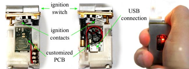
**Figure 3:** The *UbiLighter* v.2's internal buildup. The ignition contacts as read by the micro-controller are highlighted. On the left-hand side the battery compartment and LEDs are visible. The center shows the RTC, USB connector and microcontroller. The right-hand side shows that the lighter while being used operates very much like the traditional lighter.
