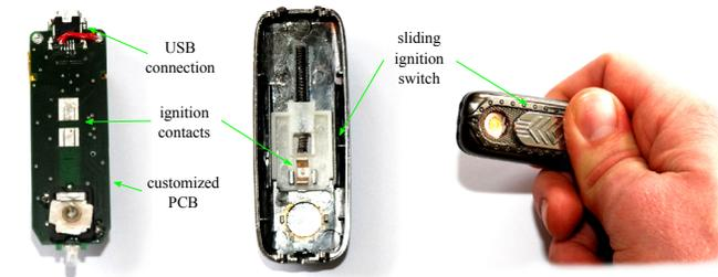
**Figure 2:** The *UbiLighter* v.1's internal buildup. On the left, a mechanical switch closes the circuit between battery and a coil, allowing it to heat up so that a cigarette can be lit up. The time and duration for which the switch was used is logged by an on-board micro-controller that is connected to a real-time clock. The right-hand side shows the lighter while being used.
