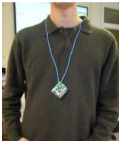
Figure 1: The Pendle is a wearable designed as mediator between user and proactive environment. It holds personal information to implicitly trigger proactive behaviour in the environment, and it provides a gesture-based interface for the user to explicitly modify the environments behaviour.
