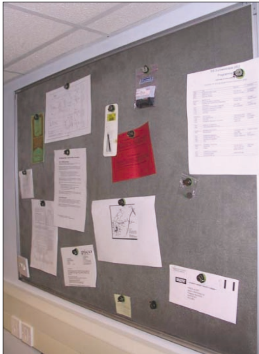
Figure 3. A working example of the networked notice board application. All pins are connected to the network bus, and generate an interrupt as soon as they meet their expiration date and time. They are powered by the notice board as well.
