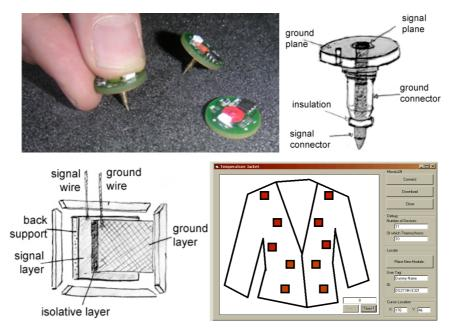
Fig. 3. The components of Pin&Play: top: the node with pin connector, bottom-left: the surface structure (using conductive textile), and bottom-right: an application using clothing as the surface and temperature measuring pins that have been attached ad hoc to the clothing [12] [9].
