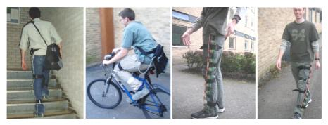
**Fig. 6.** Experiments of [10] with networks containing a large amount of motion sensors: the left two using 40 accelerometers, the right two using 90 tilt switches.
