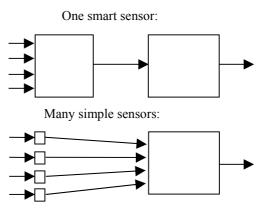
Fig. 5. Two sensor architecture approaches.
