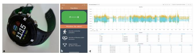
**Fig. 1** A The proposed components: data is collected and forwarded by an open-source smartwatch (Bangle.js), with our customized firmware (a) and smartphone app (b), providing a transparent data pipeline to a back-end server database for anonymized storage and inspection of all data across participants (c)
