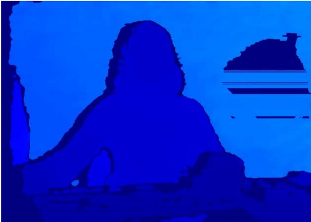
**Figure 4: A single frame from the depth camera in our setup, pointed towards the operator, which can also be used to detect breathing patterns from the chest's movements [10]).**
