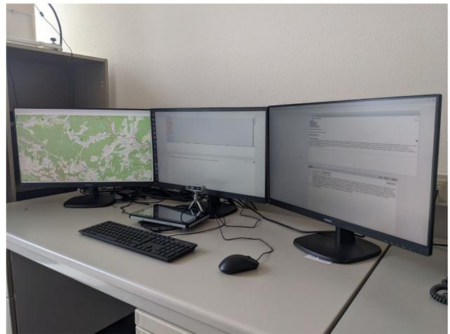
**Figure 3: Our LSTSim-based simulation setup, following a similar single user setup across three large desktop screens with a central touch screen. Study volunteers were monitored and recorded through wearable sensors, a depth camera below the screens, and simulation-internal parameters and interactions.**
