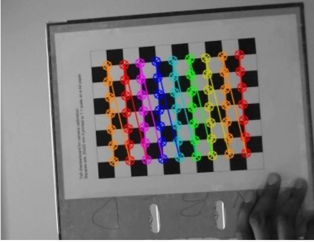
**Figure 2: The calibration process is done with a chessboard image, here is the output of the process where the corners in one of the two images are found.**
