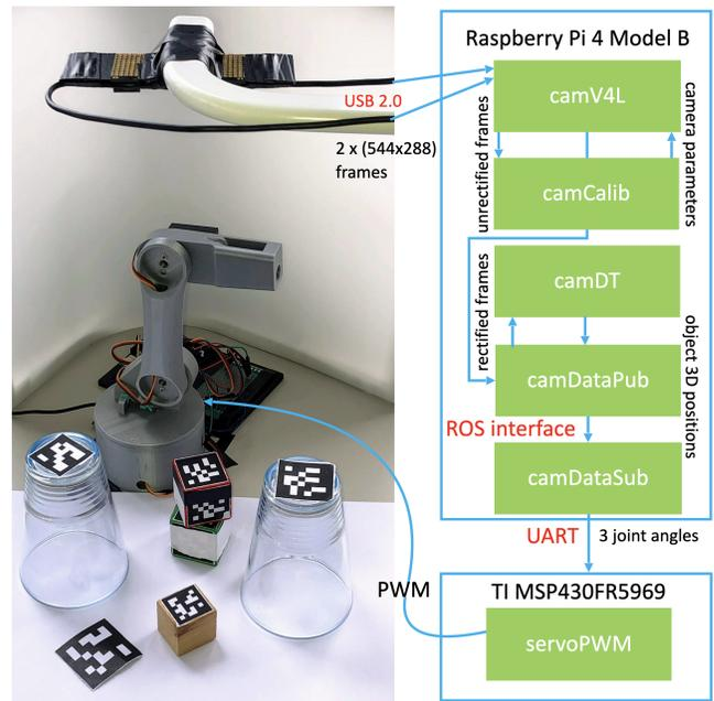
**Figure 1: Overview of the tracking and actuation parts of our prototyping framework: Two miniature web cameras provide their frames via USB to the Raspberry Pi 4B, which via OpenCV libraries uses these to perform 3D object tracking. Tracked objects are then merged in the robot's coordinate systems via ROS and can be manipulated by changing the robot arm's joints, which are sent to a microcontroller that maps the joint angles to pulse width modulation (PWM).**
